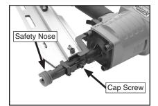
Figure 6. Loosening cap screw for depth adjustment.
